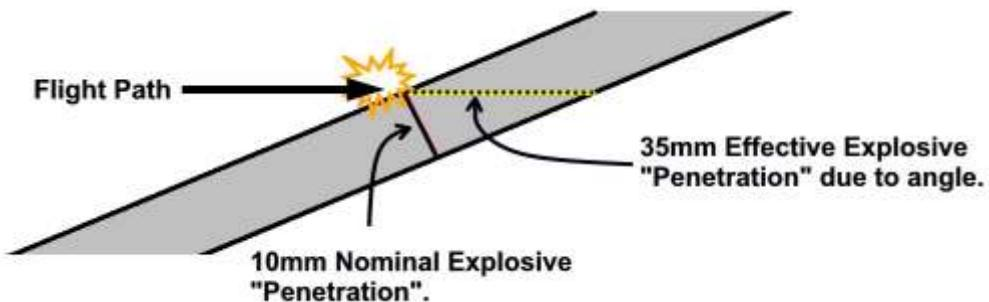
Figure 359: Effective vs. Nominal Penetration for an explosive charge.
