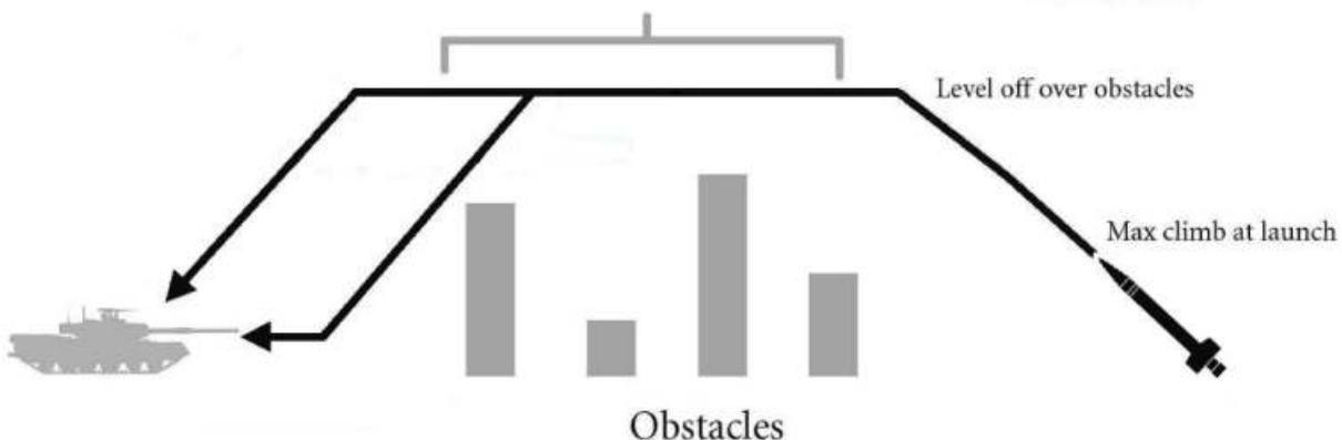
Figure 352: Powered In-flight units follow simple flight paths. If the in-flight munition is guided, the flight path is periodically adjusted to account for target movement.
