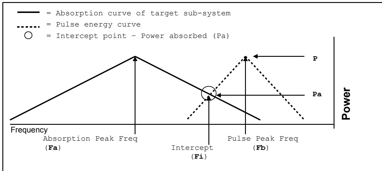
Figure 363: Coupling calculation of energy transferred between an incoming energy pulse and a target system.
