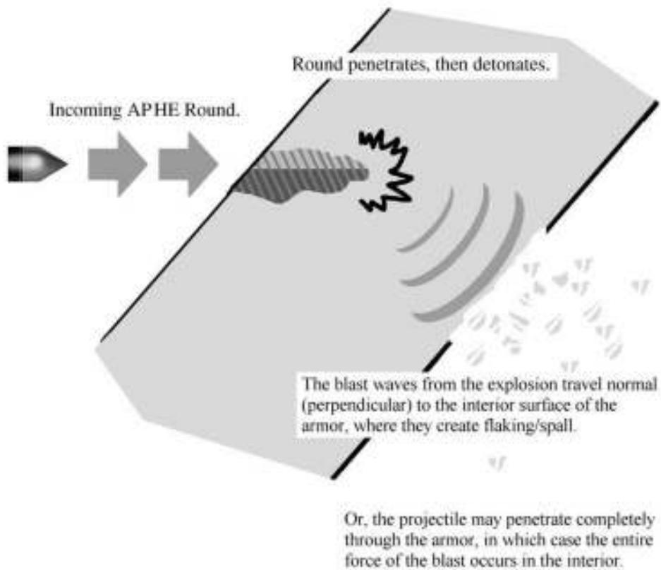
**Figure 360: APHE (Armor Piercing High Explosive) projectile fundamentals.**
