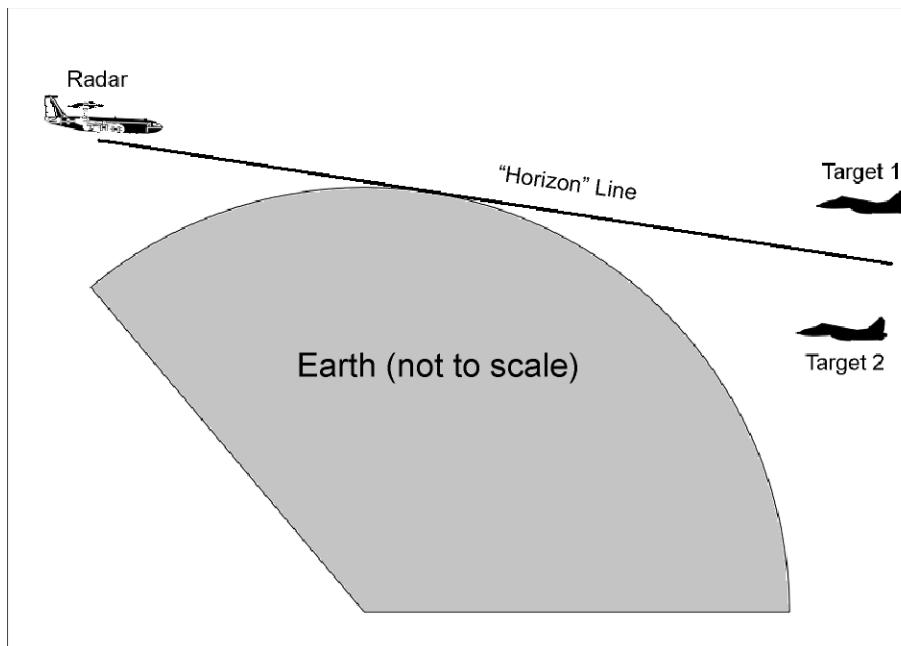
**Figure 388: The Earth's horizon blocks radar. Radars without OTH capabilities would only be able to detect Target 1. Those with OTH capability would be able to detect both. The horizon calculations include the radar and target heights above ground level (AGL).**
