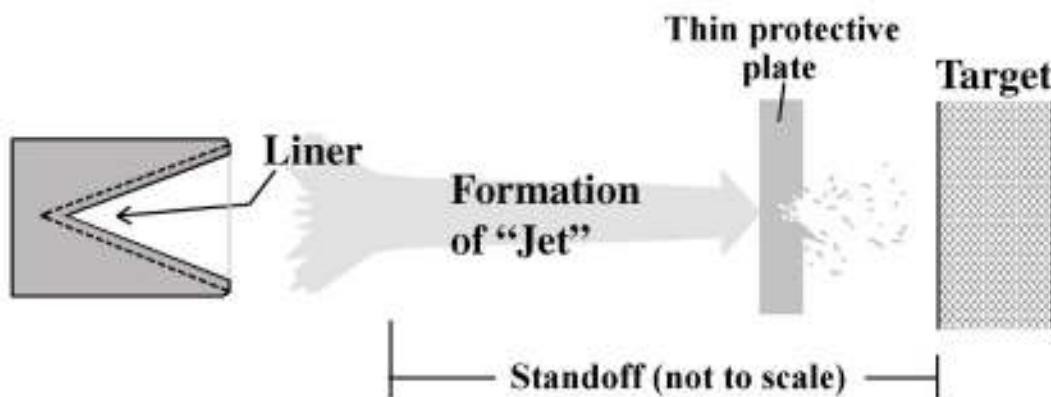
Common countermeasure - thin protective plates cause premature detonation of the warhead outside the optimal standoff.
