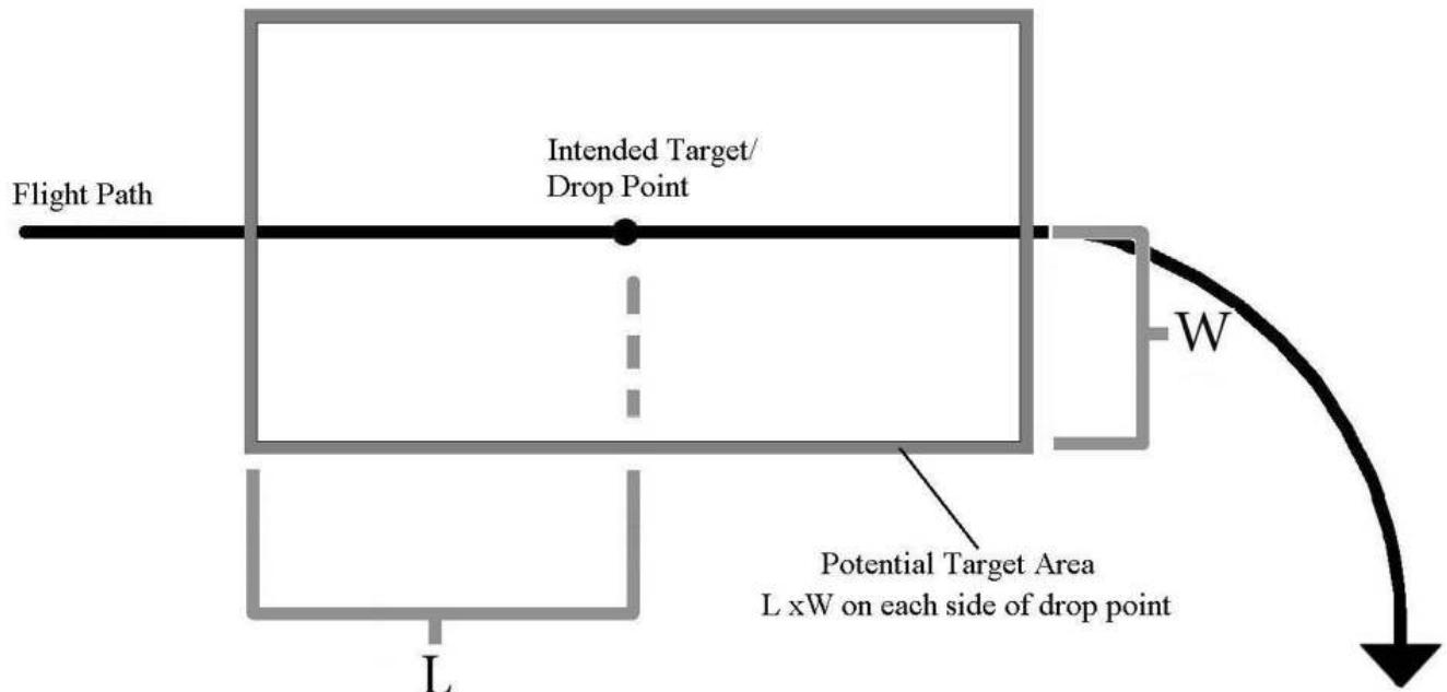
W = 100 meters for each 1000 meters of aircraft height at weapon drop (Maximum = 1000 meters).
