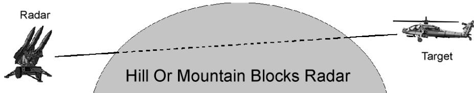
**Figure 387: The effects of elevated terrain on radar detection.**
