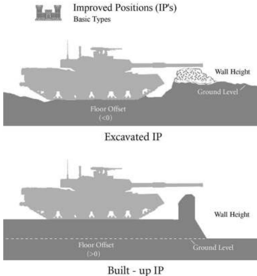
**Figure 365: Basic IP (Improved Position) Types - excavated vs. built-up.**
